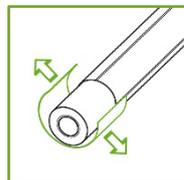
**04.** Peel back the cut section of the casing pipe.
