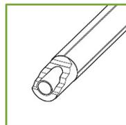
**05.** Carefully remove the PU insulation foam from the service pipe, by using a putty knife.
