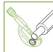
**06.** To make the pipe end straight, cut 30mm of service pipe with a suitable pipe cutter.
