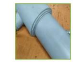
Visible check Two beads (of pipe and fitting) are visible. Correct alignment of pipe and fitting. Marked insertion depth is visible.
