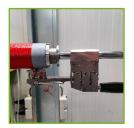
b) Remove the oxygen barrier with our Flexalen PB EVOH Scraper up to the marked insertion depth (should remain visible).
