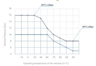
Up to OD110 20°C/16 bar 95°C/8 bar
