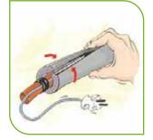
Fix the cable according to the application table (bottom of the pipe, parallel or spiral), secure on the entire length with PVC tape.
