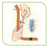
Place the thermostat (built in to ThermaLint, sensor for TracingSet) at the coldest part of the tube. For plastic pipe: always apply aluminium tape on the pipe under the heating cable.
