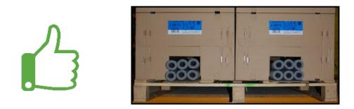
The picture above demonstrates the only correct way of opening the Thermaflex box. Any other way of opening during storage risks causing damages to the box and insulation material, due to high compression for example.
